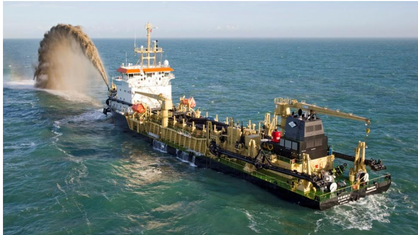
Trailing Suction Hopper Dredger
