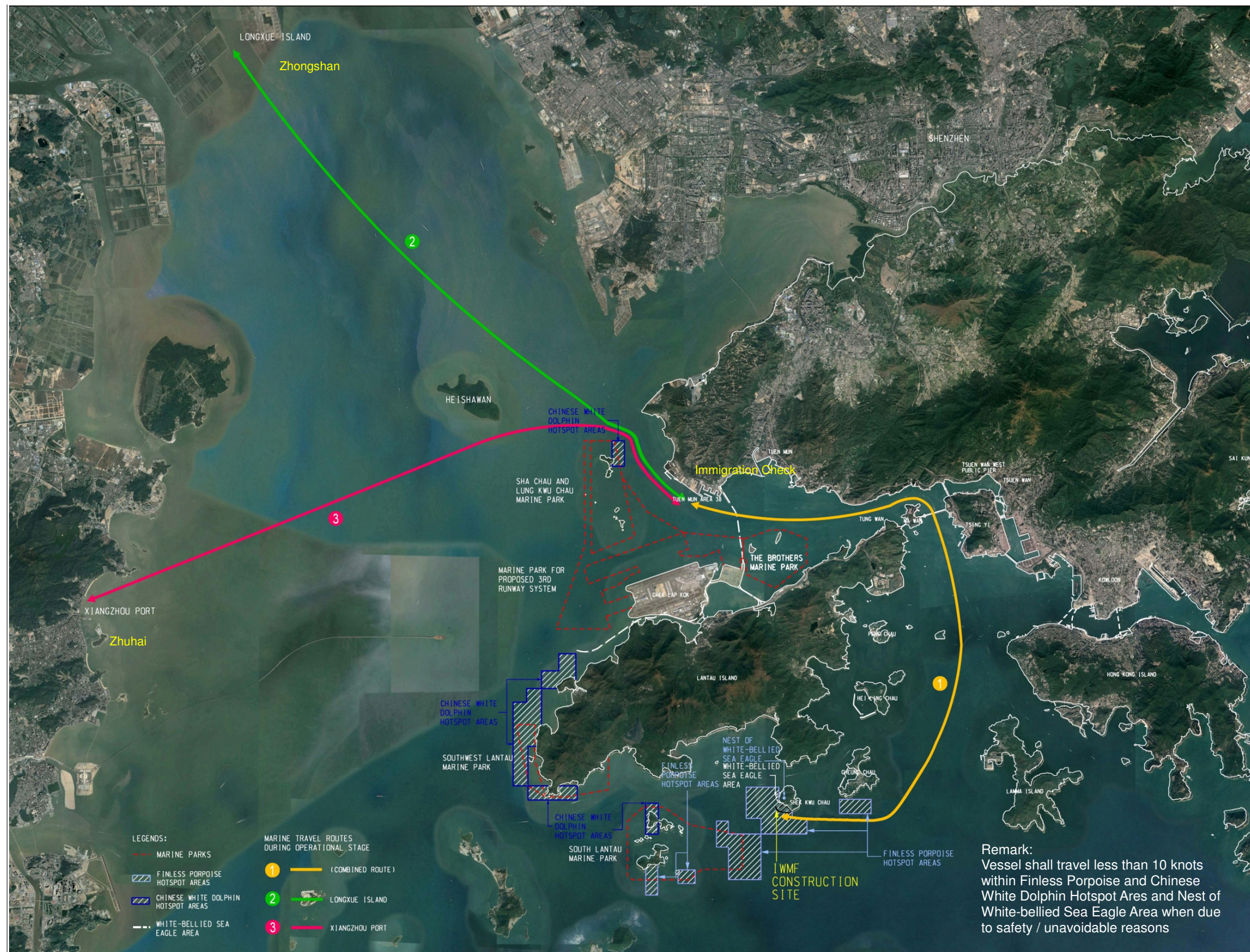
Figure 5 Marine Travel Routes for delivering Sand Fills from Zhongshan / Zhuhai, Guangdong to the construction site
