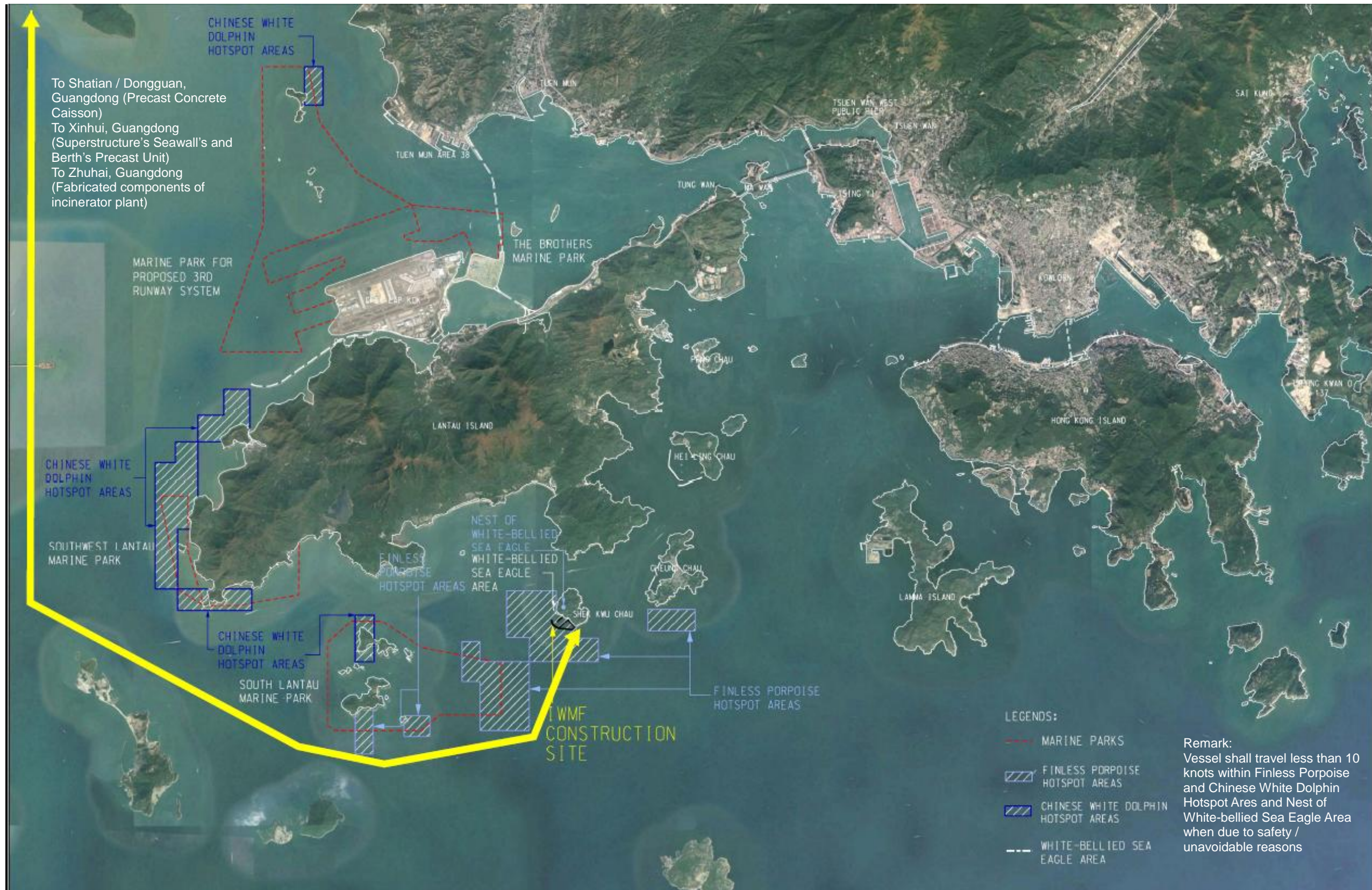
Figure 6 Marine Travel Route for delivering Precast Concrete Caisson, Superstructure's, Seawall's and Berth's Precast Unit and Prefabricated components of incineration plant to the construction site
